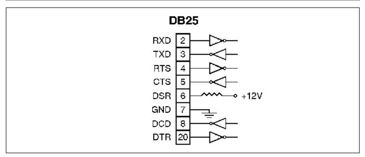
Figure A.2: Modem Port Interface (DCE)
